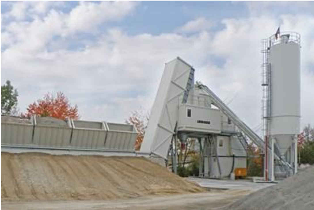
Diagram 5.3: Liebherr Mobilmix 2.5-C 115m 3 /hour Mobile Batching Plant
