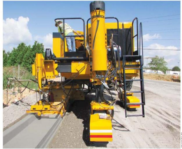
Intelligent All-Track Positioning (ATP) on the GOMACO Commander IIIx includes a smart hydraulic cylinder on each of the three legs. The smart cylinders allow G+ to know the position of all three tracks and make steering adjustments as needed.
